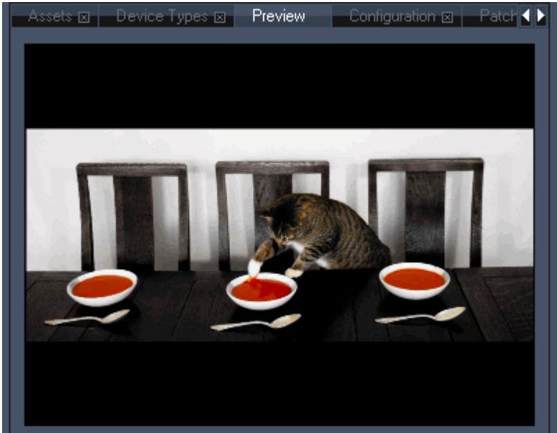
Figure C: Layer Aspect Ratio is set to "Horizontal Fit", the files aspect ratio is kept and it fits horizontally into the layer.
