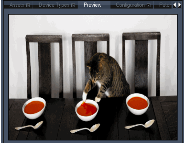
Figure B: Layer Aspect Ratio is set to "None" and the image is scaled to a 4:3 layer.
