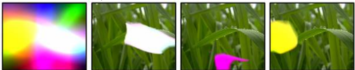
C-MIX1: Red C-MIX2: Green C-MIX3: Blue Inverted RGB colourkey based on colour selection with colourmix channels. 0.25 Softness.
