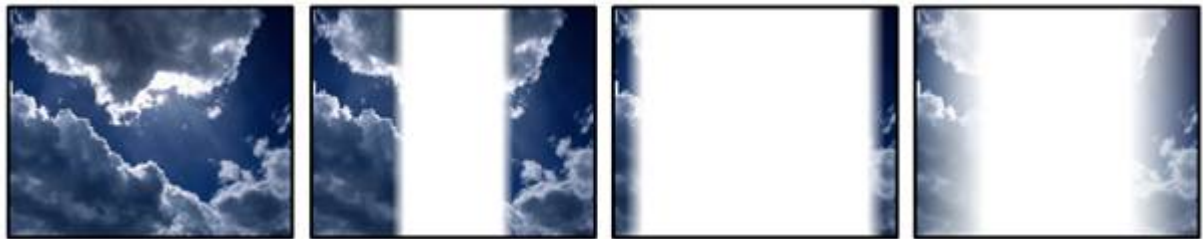
FX1: Amount FX2: Size FX3: Softness Border from center to left & right. Size and edge of border are adjustable, border is white.
