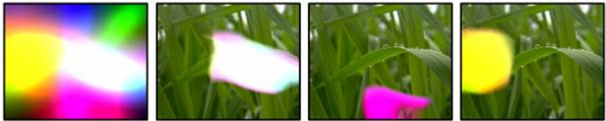
C-MIX1: Red C-MIX2: Green C-MIX3: Blue Inverted RGB colourkey based on colour selection with colourmix channels. 0.5 Softness.
