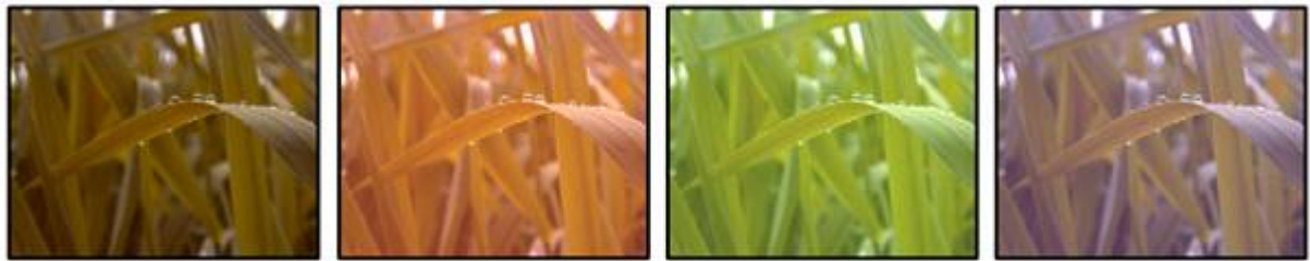
C-MIX1: Red C-MIX2: Green C-MIX3: Blue All RGB channels are shifted and added by the colourmix value.
