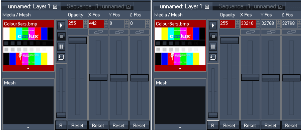
Figure 1: Fader values appear in centered position (left side) or in non-centered position (right side)
