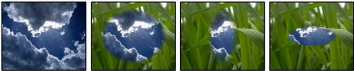
FX1: Aspect FX2: Size FX3: Softness Centered iris; shape, size and edge are adjustable. Area outside of iris is transparent.
