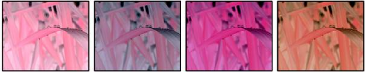
C-MIX1: Red C-MIX2: Green C-MIX3: Blue All RGB channels are shifted and added by the colourmix value plus inverted.
