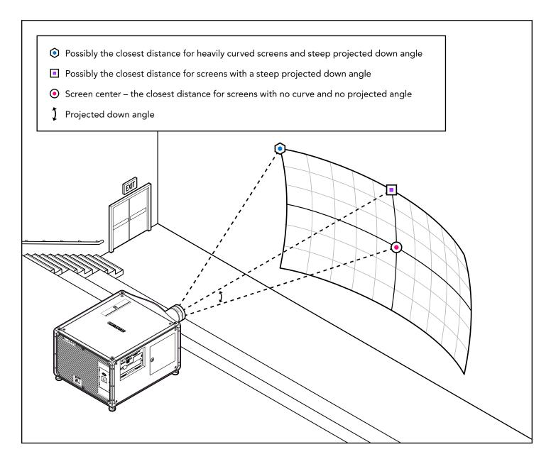
Examples of how the throw distance can be different from lens to screen center depending on projected angle and screen curve.
