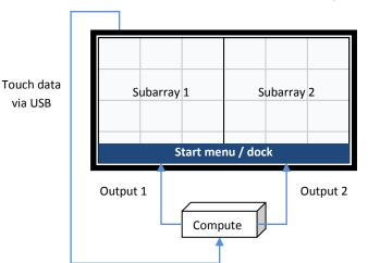
6x4 MicroTiles divided into two 3x4 subarrays
