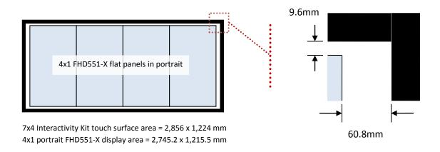
Note: When the display area is smaller than the active touch surface area, use the masking function built into the Christie Interactivity Kit to ensure touch data are mapped properly to the display. See question 3.7 below for more details.
