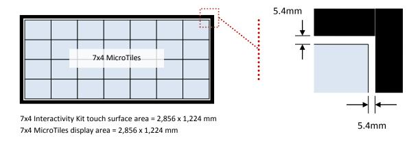
If an alternative display is being used, the size of the gap will vary depending upon the display and configuration. In some cases, the gap may be relatively large, and care should be taken to plan an aesthetic or functional way to hide or integrate the gap into the overall design. An example is provided below:
