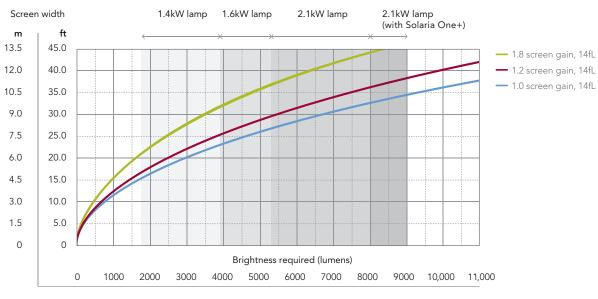
▲ Leveraging three high performing lamp options, the Christie Solaria One and Solaria One+ deliver superior brightness in the DCI color space.
