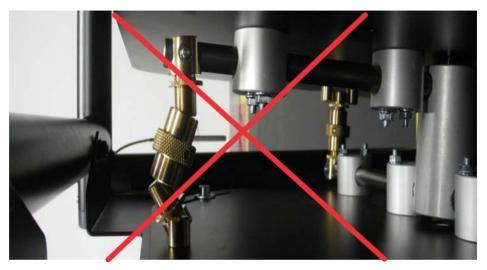
The limiting range pins on the frames help to prevent over adjustment and keep adjustments in the useful range. For pitch and yaw, ensure the gap between the pin and the plate is more than 0.5 mm. Refer to the appropriate rigging frame instruction sheet for a diagram of the adjustment pins.
