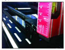
8. Adjust the bottom knob of the adapter bracket to achieve a 10 mm (0.39") gap. If further adjustment is required, leave a 1 mm (0.04") minimum clearance to allow the bracket to be easily released.
