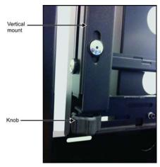
11. Check that the mount is level. If necessary fine adjust the vertical position.
