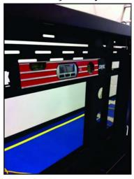
12. To avoid damage to the display, leave a minimum 1 mm (0.04") gap so the weight of the panels do not rest on the panels underneath. It may be necessary to re-adjust the vertical position to prevent this.
