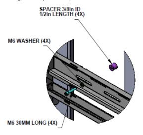
6. Tighten the wall mount to the F100 Frame using the four M6 screws. Never tighten in excess of 80 in-lbs (9 Nm).
