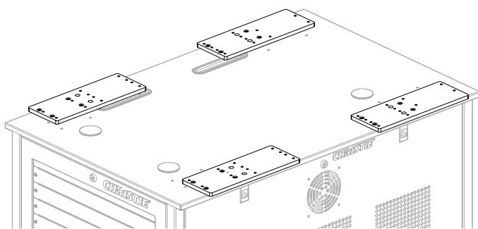
2. Install four screws for each front plate and keep the screws loose.
