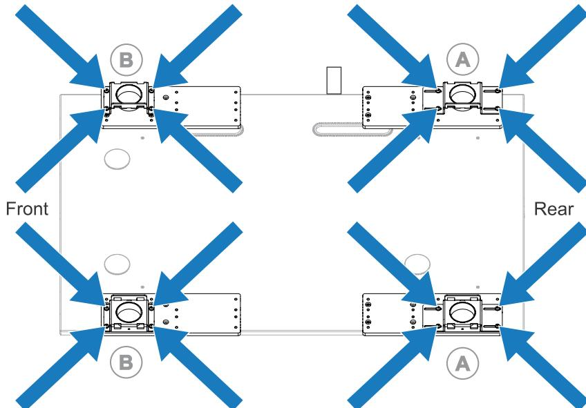
5. Install four screws for each holder and torque only the front foot holder screws.
