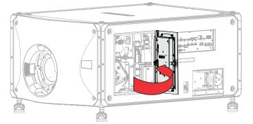
3. For Sapphire 4K40-RGBH, disconnect the intelligent filter holder harness on the optical filter ID (OFIB) board.
