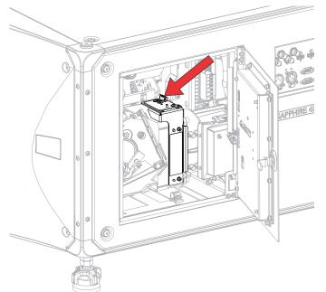
4. Wearing gloves, remove the two screws securing the existing optical filter and remove and store it.
