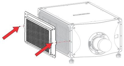
5. Unbag the filter and install the filter by sliding it in the open slot of the frame by compressing the spring tab, making sure to adhere to the air flow direction marked on the filter (highlighted by the blue arrow in the image below).
