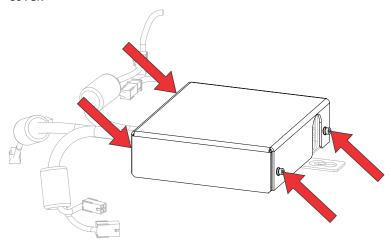
5. Loosen the screw securing the board to the bottom enclosure.
