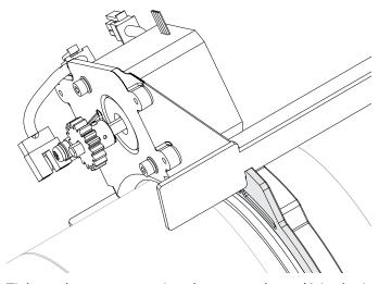
7. Tighten the screw securing the motor clamp (A in the image below).
