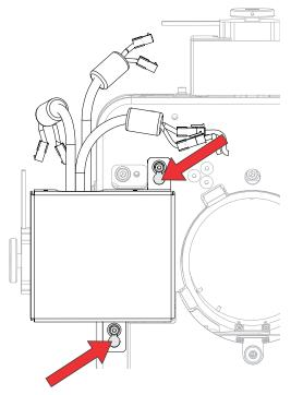
4. Remove the four screws securing the top cover of the motor control assembly and remove the cover.
