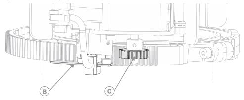
11. Loosely clamp the gear clamp into place until it is placed against the bottom of the position plates.
