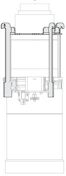
6. Adjust until the motor clamp is seated on the shoulder position plates.
