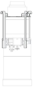
6. Adjust until the motor clamp is seated on the shoulder position plates.
