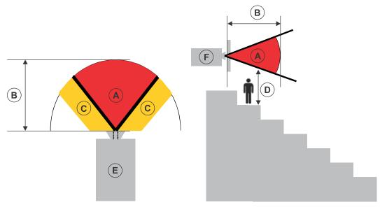
• A—Hazard zone. The region of space where the projection light from the projector is above emission limits for Risk Group 2. The light intensity may cause eye damage after a momentary
