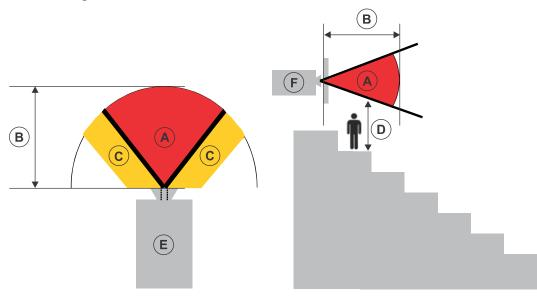
B—Hazard distance. Operators must control access to the beam within the hazard distance or install the product preventing potential exposure of the spectators' eyes from being in the hazard distance.
