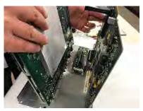
14. To hold the IMS3000 in place, engage the support bracket.
