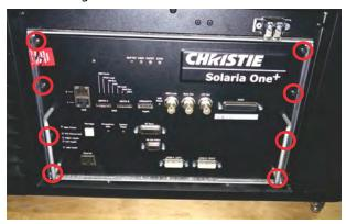
5. Using the two handles, pull the card cage faceplate assembly out of the card cage.
