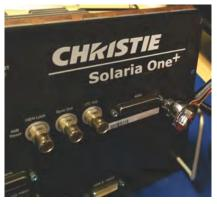
9. Using a 2.5 mm ball hex driver, remove the left screw securing the Christie IMB to the faceplate. Set the screw aside.
