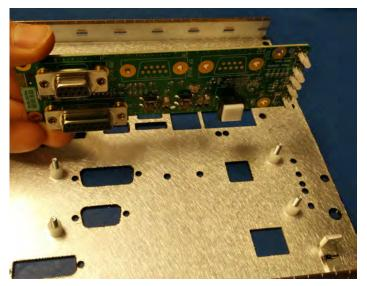
5. Secure the PIB faceplate board to the faceplate using the four nuts set aside in step 18 of the disassembly procedure. Torque the nuts to 10 in-lb.
