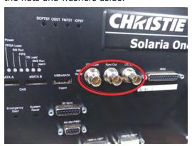
8. Using a 3/16 nut driver, remove the two nuts on either side of the AES3 output. Set the nuts aside.
