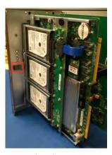
16. Using the three HDBNC nuts and six #1 Phillips screws provided with the IMS3000 kit, secure the IMS3000 board to the faceplate.
