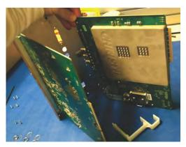
14. Using a 3/16 nut driver, remove the 3D Sync, RS 232 PIBS1, HDMI A/LEFT, and HDMI B/RIGHT nuts. Set the nuts aside.
