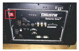
4. Using a #2 Phillips® screwdriver, remove the eight screws securing the card cage faceplate to the card cage. Set the screws aside.
