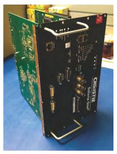
7. Using a 14 mm wrench or deep socket, remove the GEN Lock, Sync Out, and LTC Out nuts. Set the nuts and washers aside.
