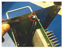
12. Using a 2.5 mm hex driver, remove the two screws on the bottom of the PIBS1 board. Set the screws and support bracket aside.
