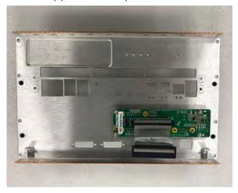
6. Install the EMI gasket provided with the Dolby IMS3000 to the faceplate, as shown.
