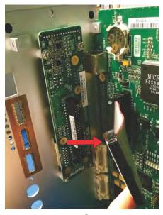
16. Using a #1 Phillips $^{\$}$  screwdriver, remove the two screws securing the PIBS1 board to the faceplate. Set the screws aside.
