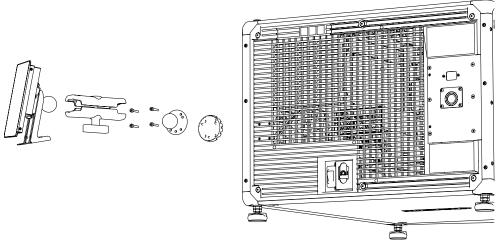
Install the spacer on the rear cover.
