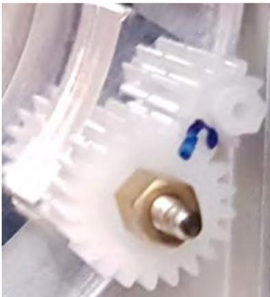
2. If the boresight screws are not in their initial position, turn the screws counterclockwise until they stop and then turn the screws clockwise until the blue marks are aligned as shown above.
