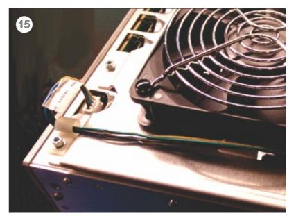
15. Obtain the 120 mm fan bracket assembly from the fan upgrade assembly kit #003-006817-01, attach it loosely using the seven screws (previously removed) and install the p-clip from the upgrade kit. Torque all screws to 8 in-lb and thread the fan harness through the p-clip as shown on tag 15. Connect the harness to the plug and flex it up as shown in the photograph.
