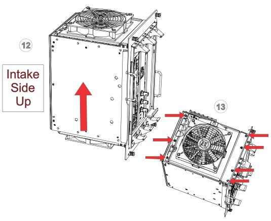
13. Remove the seven 2.5 mm hex screws shown on tag 13 graphic above and disconnect the fan wire located between the lower two left-hand fan bracket screws.
