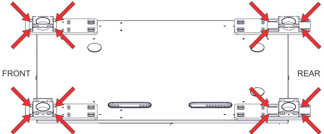
5. Install four M5 screws for each holder and torque only the front foot holder screws.
