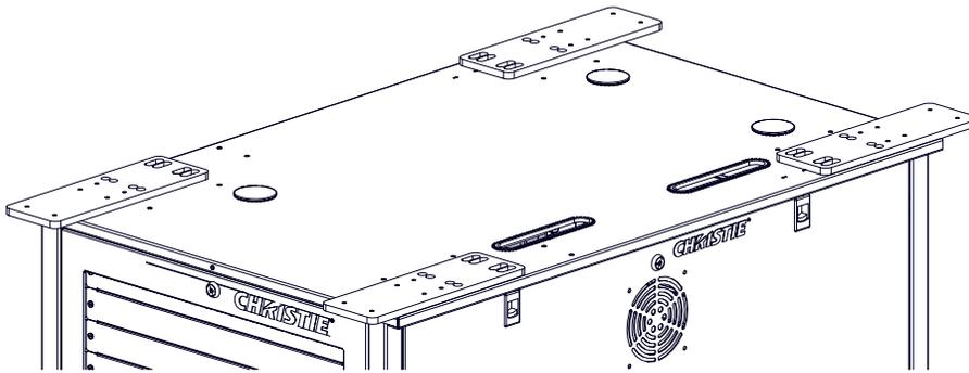
2. Install two M5 screws for each front plate and keep the screws loose.
