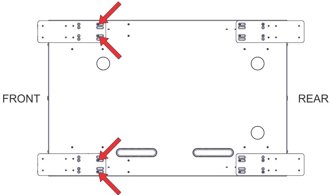
3. Install four M5 screws for each rear plate and torque the screws.
