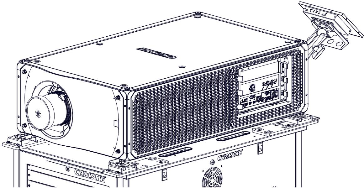
7. Install the foot cover bracket on all the feet and torque the four screws.
