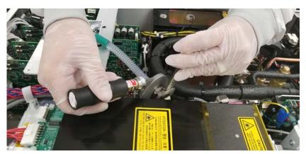
13. Connect the other end of the new hoses to the chiller. Note the routing of the coolant hoses in the photo below.
