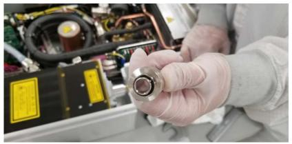
12. Install the new hoses on the LOS. Torque to 20 in-lb.
