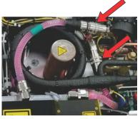
6. Loosen the four locknuts to release the Light Optical System (LOS).
