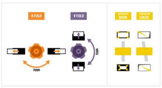
Refer to the test pattern for guidance on making the adjustments. The right panel of the test pattern provides information about the integrator zoom and focus adjustments. The left panel provides information about the fold mirror adjustments.
