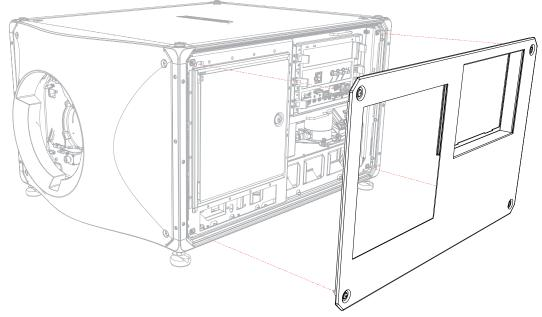
2. Remove the electronics-side cover.
