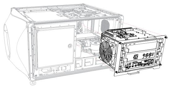
9. Pull on the locking pin and slide the card cage out along the guides.
