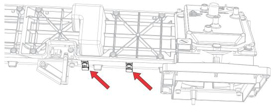
6. Remove the six screws securing the integrator assembly.
