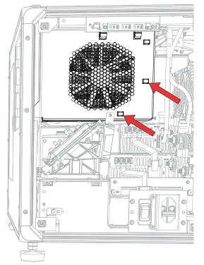
2. Remove the five screws securing the rear card cage security bracket.
