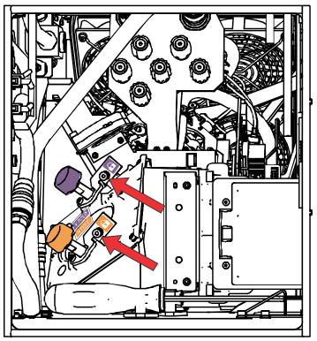
8. To make horizontal adjustments on the fold mirror, use the orange adjustment knob. To make vertical adjustments on the fold mirror, use the purple adjustment knob.
