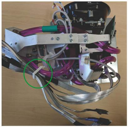
When complete, the light engine should resemble the photograph below:
