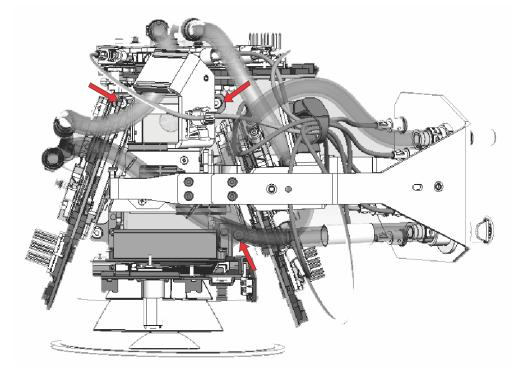
Tighten the screws to 15 in-lb to ensure the light engine does not become detached from the base plate during transportation.
