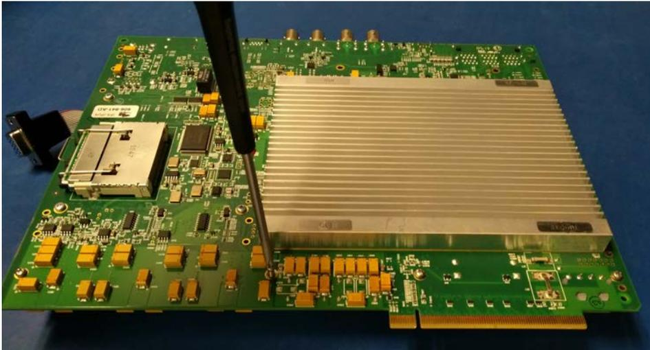
26. Install the long 4/40 stand-off provided in the conversion kit. Torque the stand-off to 8 in-lb.
