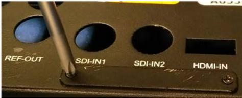
8. Using a 7/32 nut driver or pliers, remove the four nuts securing the two SATA harnesses to the faceplate. Set the nuts aside.
