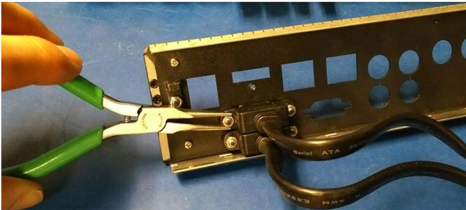
9. Using a flat head screwdriver, remove the two SATA harnesses from the faceplate. Set the harnesses aside.
