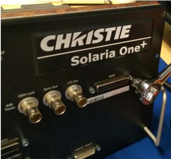
9. Using a 2.5 mm hex driver, remove the left screw securing the Christie IMB to the faceplate. Set the screw aside.
