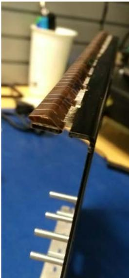
14. Pull the long flange of the EMI gasket over the edge of the faceplate.
