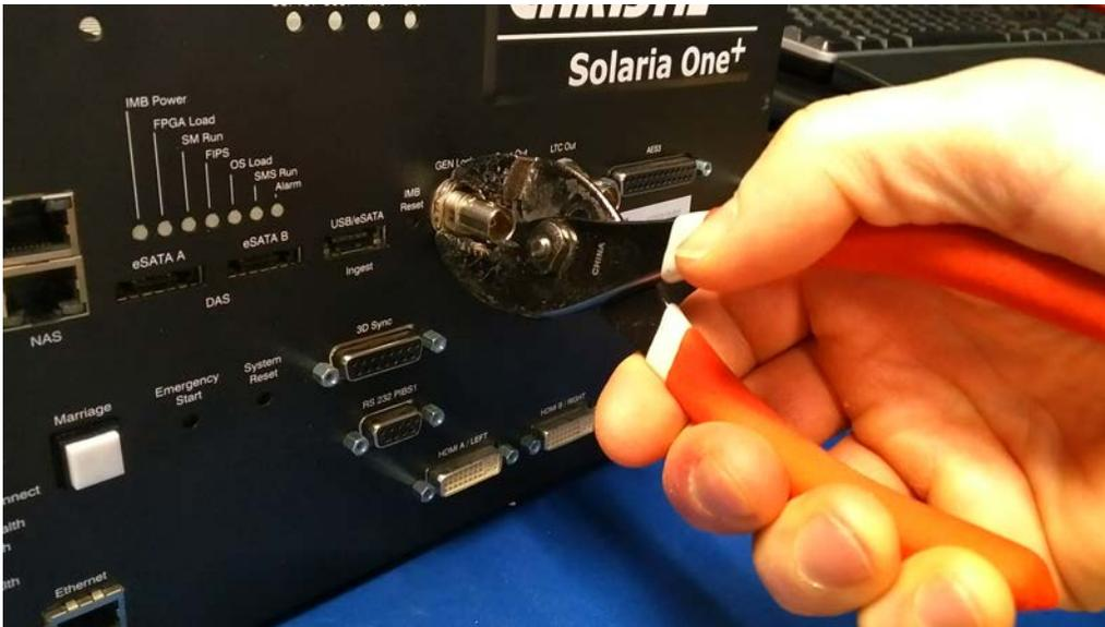
8. Using a 3/16 nut driver or pliers, remove the two nuts on either side of the AES3 input. Set the nuts aside.
