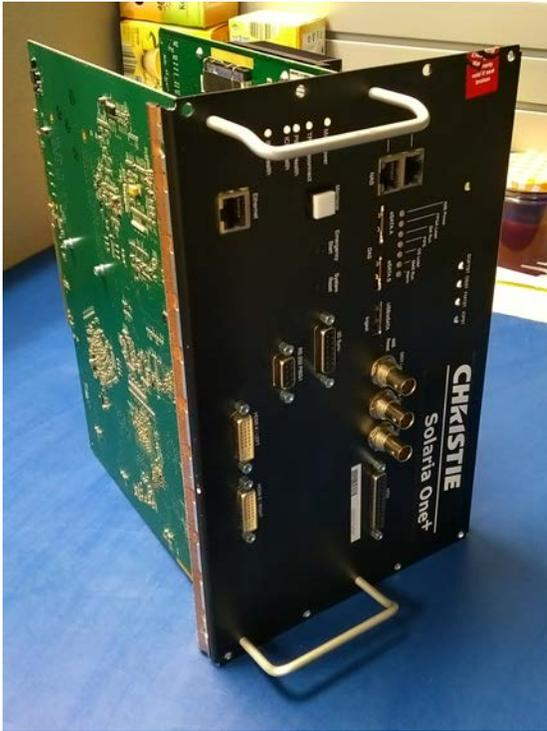
7. Using a 14 mm wrench or pliers, remove the GEN Lock, Sync Out, and LTC Out nuts. Set the nuts and washers aside.
