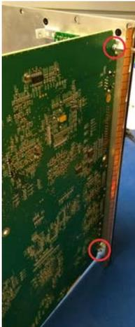
17. Carefully separate the PIBS1 board from the faceplate. Set the board aside.
