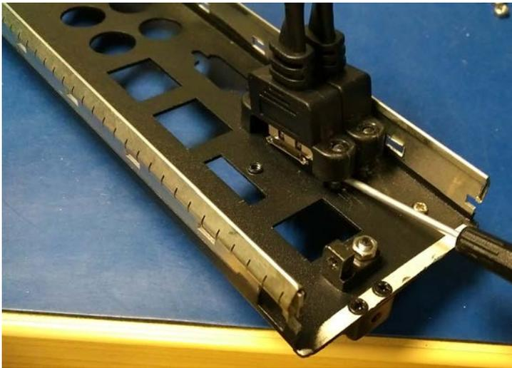
10. Using a 7/32 nut driver or pliers, remove the two nuts securing the mounting brackets to the faceplate. Set the nuts aside.
