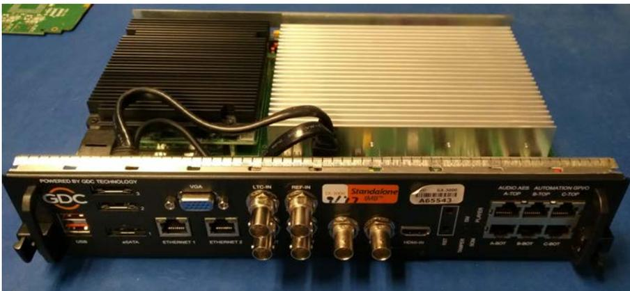
2. Using a #1 Phillips® screwdriver, remove the two screws securing the SX-3000 board to the SX-3000 faceplate.
