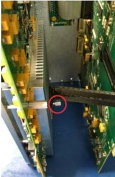
35. Using the handles and #1 Phillips® screws removed in step 19 of the disassembly procedure, install the handles onto the faceplate. Torque the screws to 6 in-lb.
