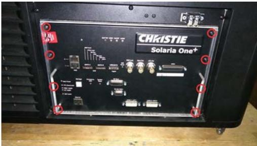
5. Using the two handles, pull the card cage faceplate assembly out of the card cage.
