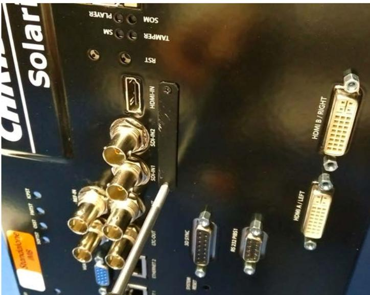
37. Install the card cage faceplate assembly in the projector.
