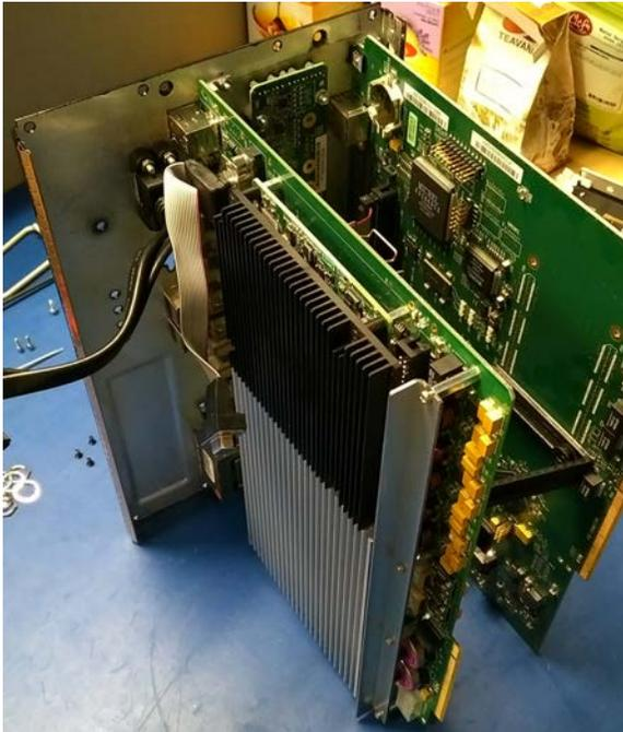
29. Install the two LTC nuts, two REF nuts, and two SDI washers and nuts removed in step 6. Torque the nuts to 8 in-lb.
