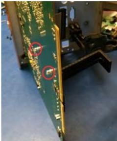
25. Using a #1 Phillips® screwdriver, remove the screw from the back of the SX-3000 board.
