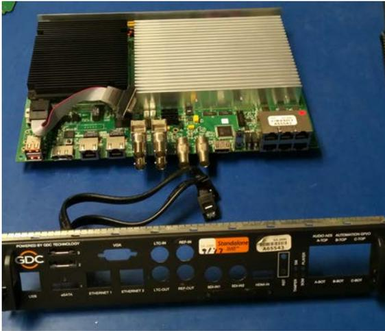
7. Using a #1 Phillips® screwdriver, remove the two screws securing the ID plate to the faceplate. Set the ID plate and screws aside.
