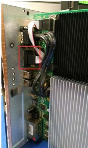
32. Insert the EMI gasket removed in step 21 of the disassembly procedure.
