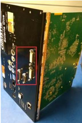
22. Using the two screws set aside in step 16 of the disassembly procedure, secure the PIBS1 board to the faceplate. Torque the screws to 10 in-lb.
