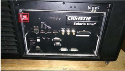
4. Using a #2 Phillips® screwdriver, remove the eight screws securing the card cage faceplate to the card cage. Set the screws aside.
