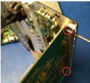
23. Torque the 3D Sync, RS 232, PIBS1, HDMI A/LEFT, and HDMI B/RIGHT nuts to 10 in-lb.
