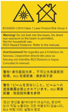
Indicates a light hazard. Do not look directly into the lens. The extreme high brightness can cause permanent eye damage.
