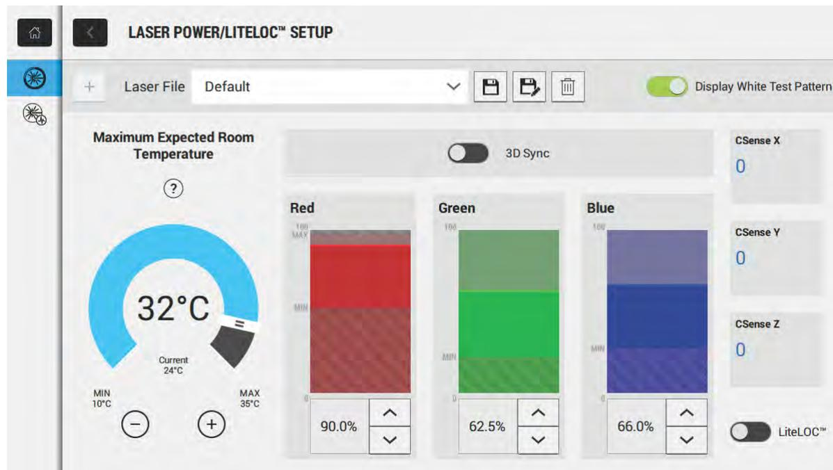
When refining the laser power settings, the amount of time required to re-stabilize the projector depends on the size of the adjustment. For very small adjustments to the expected room temperature
