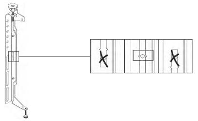
The exterior side of the bracket has the diamond and notches. When looking at the back of the display panel, the bracket in the above image should be installed on the left side of the display panel.
