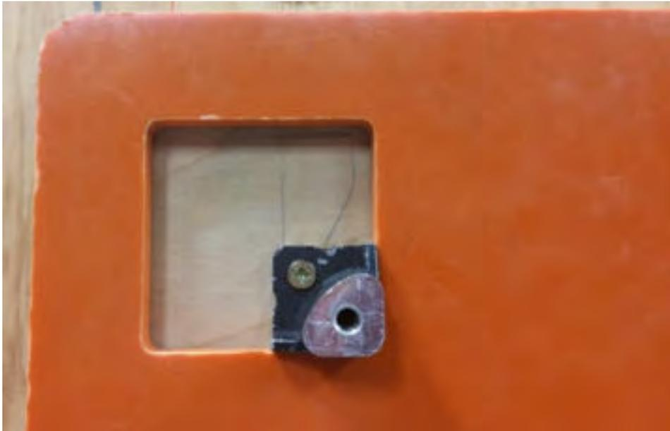
The corners and sides of the tiles should line up with the center of the mounting blocks.
