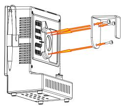
2. Slide the mounting bracket into the bracket support.
