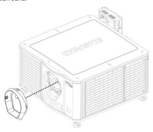
2. Turn the lens clamp on the front of the projector to the open position with a hex key.
