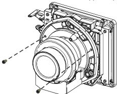
7. Lock the lens assembly in place with a hex key.
