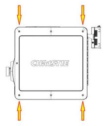
2. Position a single stacking cup (011-104349-XX) over one of the empty screw holes so the higher side of the cup faces outward and aligns with the projector skin.
