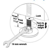
To ensure optimum performance of the projector, install the projector so it is centered and parallel with the screen. To compensate for tilt or offset, you can adjust the projector feet and the lens mount position.
