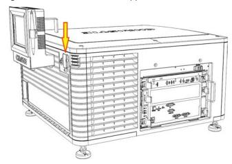
3. Connect the connector from the TPC to the port on the rear of the projector.
