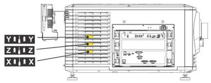
b. Insert a 5 mm hex driver through the louvers at an angle below the Y axis adjustment label until it is firmly seated on the Y axis adjustment screw.
