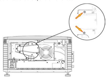
9. Loosen the two thumbscrews and open the lamp access door.
