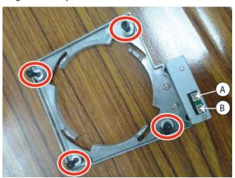
2. Install the E Series lens adapter ensuring the connector pin is facing up and is on the left-side of the lens motor.
