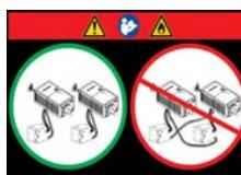
Indicates that, in a multi-projector installation, there is a risk of a fire hazard if the high current DC cables and interlock/control cables are incorrectly cross-connected between the projector heads and lamp power supplies. Make sure the high current DC leads and interlock/control cables are correctly connected between the lamp power supply (LPS) and its corresponding projector. Failure to comply may result in a fire hazard.
