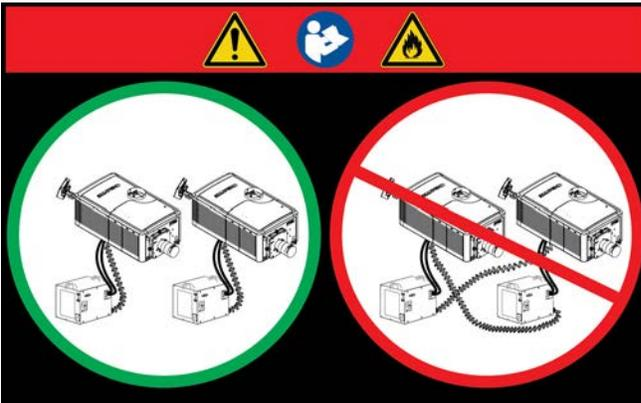
This label warns of a cross-connection hazard when installing multiple projectors at once. A fire hazard exists if a lamp power supply interlock cable is connected to a different projector than its lamp power cables.
