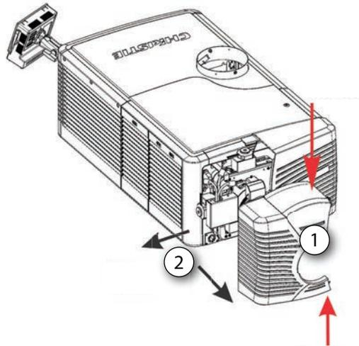
3. Place the shroud covers on a clean surface to prevent scratches.
