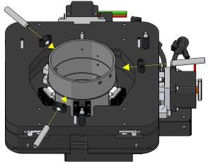
3. Tighten each locking screw until each screw contacts the lens offset collar.
