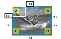
To push the mirror, turn thumbscrews counter-clockwise in zones C1-A-A1.
