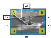
To pull the mirror, turn thumbscrews clockwise in zones C1-A-A1.
