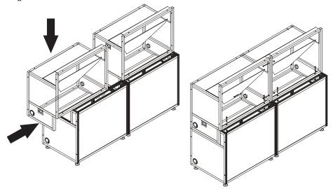
c. To secure the cube to the pedestal or cube in the lower level, use six M6 x 75 mm screws (4 for CC50) with washers and hex nuts. To allow for small adjustments, do not fully tighten the mounting hardware identified in step 1.
