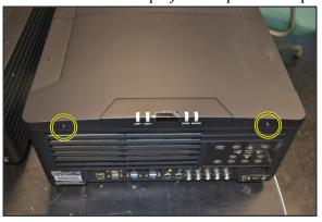
2. Remove 10 black screws from under the lamp compartment lid.
