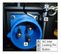
1. Remove the locking pin from the bracket surrounding the AC receptacle at the AC inlet of the projector by pressing down on the button on the end of the locking pin, and then pull upwards on the pin to remove it.
