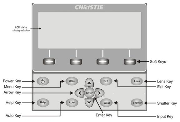
FIGURE 3-2 BUILT-IN KEYPAD
