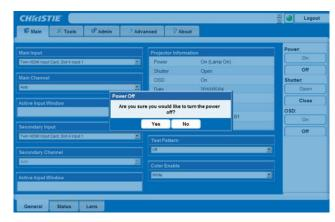
**NOTES: 1)** For Step 2 and 3, if the second key is not pressed immediately, a confirmation window will appear. The second key press must be pressed within 1 second of the window appearing. **2)** After powering down, the Status LEDs cycle and the LCD displays the message "Cooling Down", until cool down is complete.
