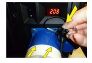
A WARNING Do not attempt operation if the AC supply and cord is not within the specified ratings. On power down, wait 5 minutes for the fans to turn OFF before unplugging the projector. Always switch off the projector before unplugging the AC line cord.
