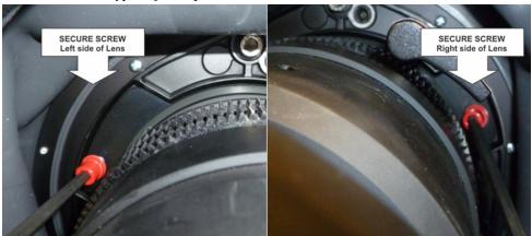
6. Use a 5mm hex driver to fasten the red security screws provided with the lens mount, or hand tighten the lens retaining screws attached to the lens.
