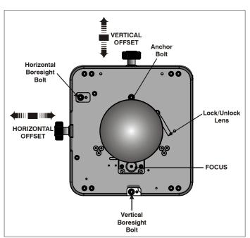
Figure 4-1 Standard Lens Mount
