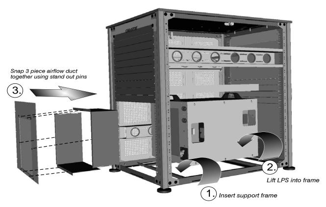
Figure 2-4 Steps to Installing LPS
