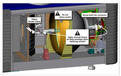
Figure 6-2 Installing the Lamp
