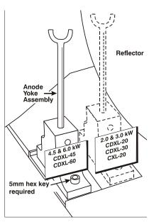
Figure 7-3 Lamp Yoke Position
