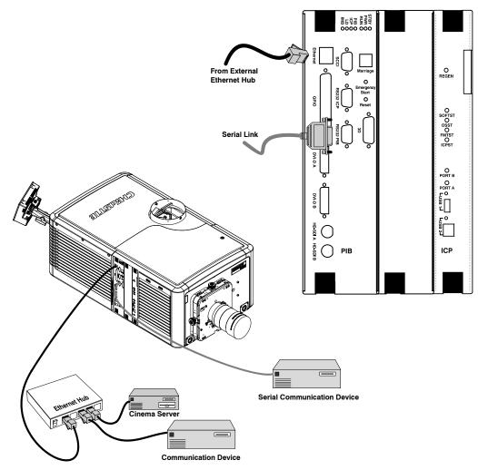
Figure 3-1 Connecting Communications
