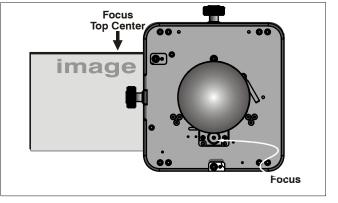
Figure 4-5 Focus Top Center of Screen
