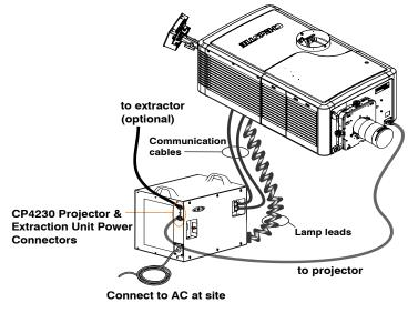
NOTE: Shroud removed for clarity Figure 2-23 LPS Connection
