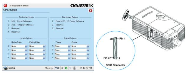
Figure 3-2 Admin: GPIO Setup Window and GPIO Port Location on cinema projector
