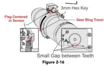
6. Turn the lens clamp to the OPEN position on the MLM and fully insert the assembly straight into the lens mount opening without turning. When the lens is fully inserted it is seated properly within the lens mount and the aperture is installed correctly.
