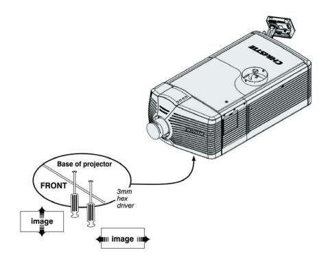
Figure 4-9 Fold Mirror Adjustment
