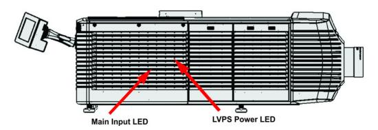
Figure 7-2 View Power Status LEDs
