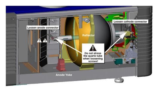
Figure 6-1 Removing the Lamp
