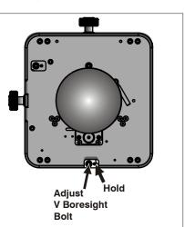
Figure 4-6 Adjust Vertical Boresight Bolt
