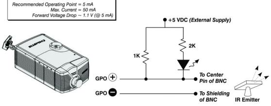
Figure 3-3 GPIO Circuit Diagram
