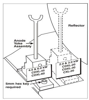
Figure 2-21 Yoke assembly installation
