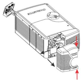
Figure 2-12 Shroud Removal
