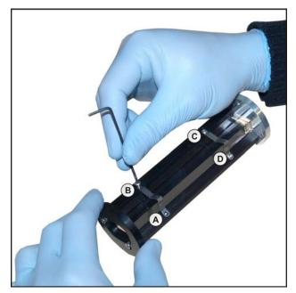
**Figure 4 Remove Existing Springs**
