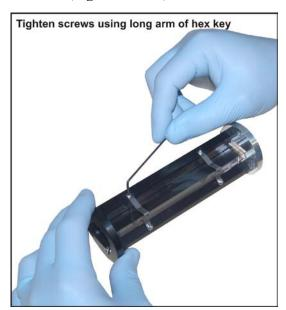
Figure 7 Secure Replacement Clips
