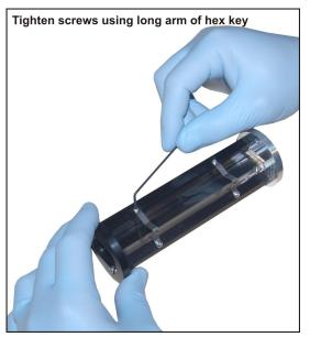
Figure 7 Secure Replacement Clips
