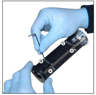
Figure 4 Remove Existing Springs
