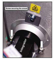
2. Carefully remove the black aluminum cover to expose the two Integrator Spring Clips (**Figure 3**).
