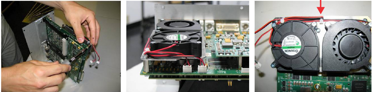
FIGURE 7 INSPECTION OF BLOWER KIT INSTALLATION
