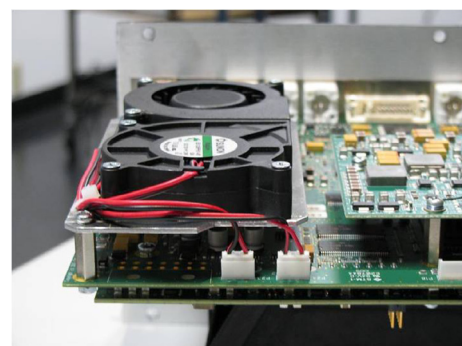
FIGURE 6 PLUG IN FAN POWER
