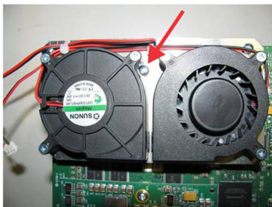
FIGURE 4 INSTALL CENTER SCREW
