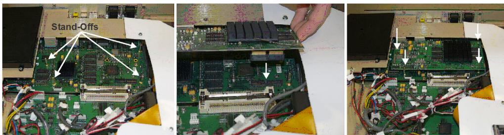
**FIGURE 5 3 CHIP XE DLP - 500W, 1.0KW & 1.2KW WARPING MODULE INSTALLATION**
