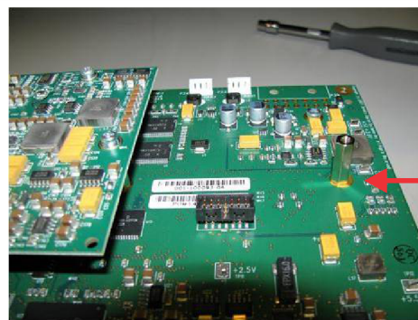
FIGURE 2 REPLACE #1 SCREW WITH 16MM STAND-OFF
