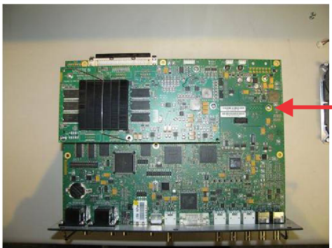
FIGURE 2 REPLACE #1 SCREW WITH 16MM STAND-OFF
