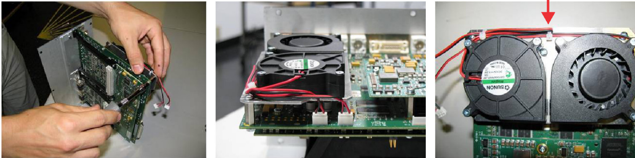
FIGURE 6 INSPECTION OF BLOWER KIT INSTALLATION
