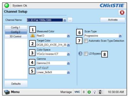
Figure 6-13 Channel Setup: Config 2 Window
