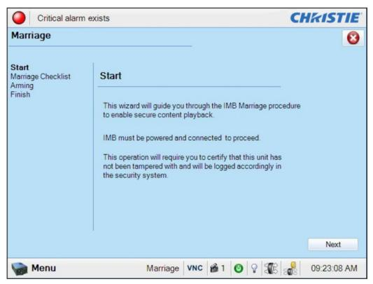
Figure 6-45 Service Setup: IMB Marriage Window
