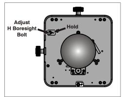
Figure 4-4 Adjust Horizontal Boresight Bolt
