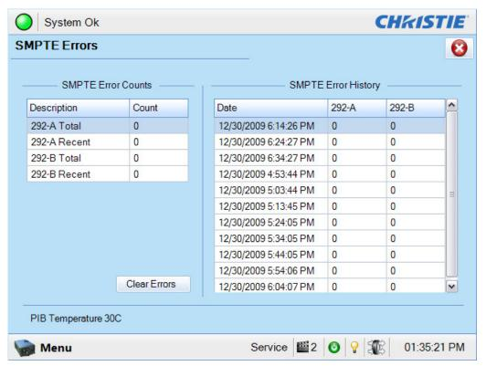
Figure 6-6 Diagnostics: SMPTE Errors Window
