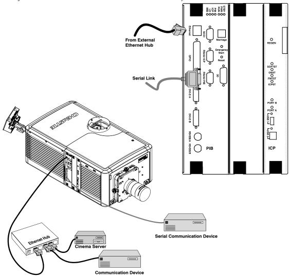
Figure 3-2 Connecting Communications
