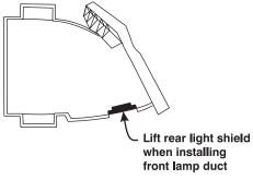
Figure 7-3 Light Shield on Front **Lamp Duct**
