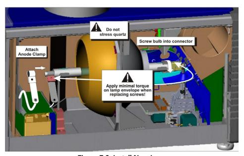
Figure 7-2 Install New Lamp
