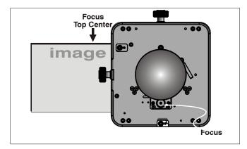
Figure 4-5 Focus Top Center of Screen
