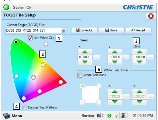
Figure 6-26 Advanced Setup: TCGD File Setup Window
