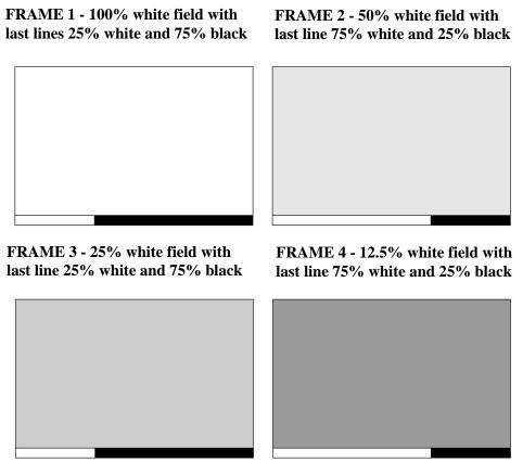
Figure 4-13 RGB-12bit-3D Half Descending Test Pattern
