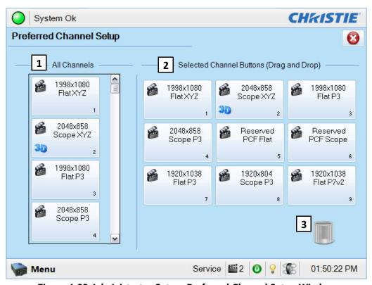
Figure 6-28 Administrator Setup: Preferred Channel Setup Window
