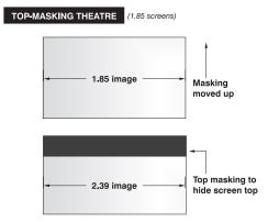
Figure 5-4 Top Masking for Scope
