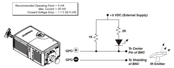
Figure 3-4 GPIO Circuit Diagram
