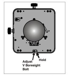
Figure 4-6 Adjust Vertical Boresight Bolt
