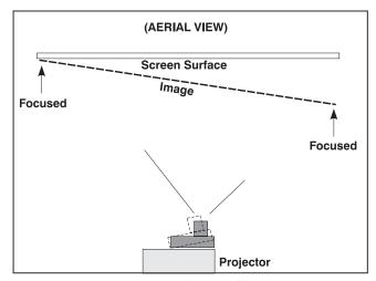
Figure 4-3 Aerial View Illustrating Misaligned Boresight
