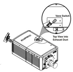
**A CAUTION** Never disable the vane switch. Attempting to operate the cinema projector with inadequate airflow can result in dangerous overheating of the cinema projector.
