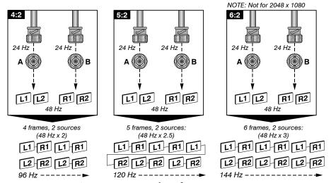
Figure 6-15 Examples of Frame Rate N:M
