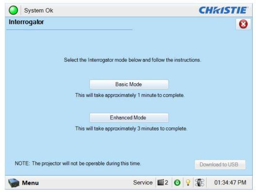
Figure 6-5 Diagnostics: Interrogator Window
