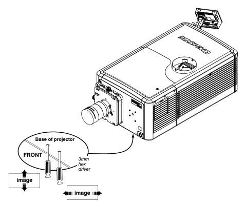
Figure 4-9 Fold Mirror Adjustment
