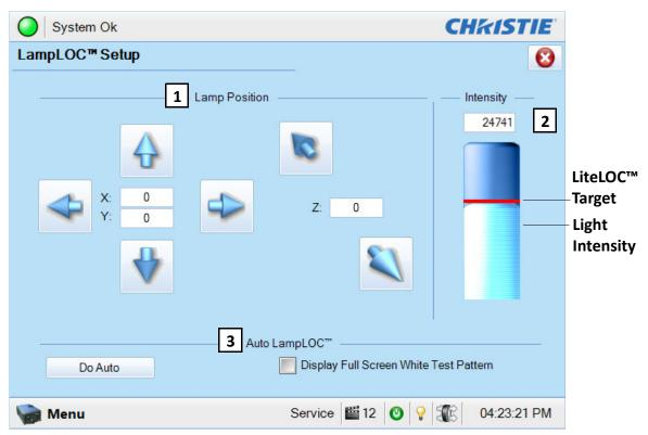
Figure 6-20 Advanced Setup: LampLOC™ Setup Window
