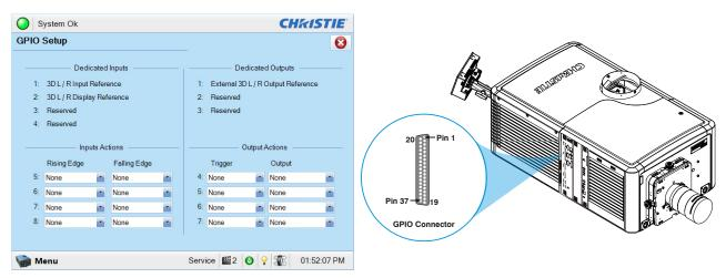
Figure 3-3 Admin: GPIO Setup Window and GPIO Port Location on cinema projector
