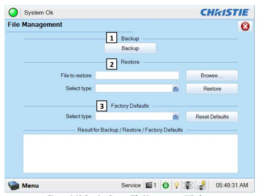
Figure 6-43 Service Setup: File Management Window
