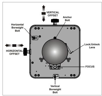
Figure 4-1 Standard Lens Mount
