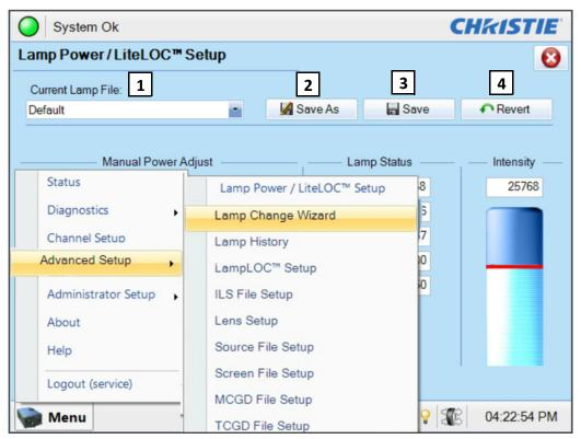
Figure 6-16 Functionality in Advanced Setup Windows
