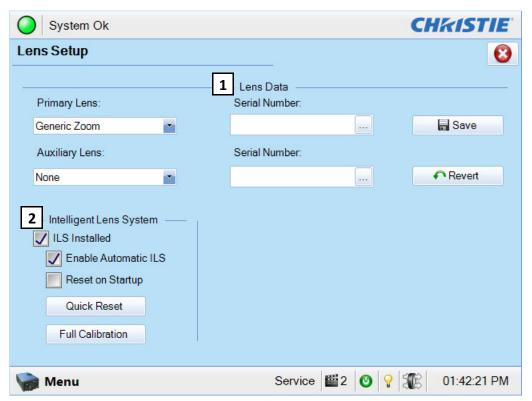
Figure 6-22 Advanced Setup: Lens Setup Window
