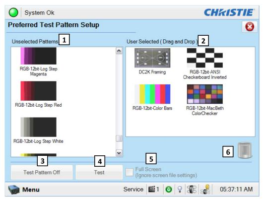
Figure 6-29 Administrator Setup: Preferred Test Pattern Setup Window
