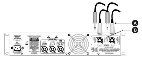
A3-pin XLR, or 6.3 mm (1/4 in.)<br/>phono jacks connected to the CH. A<br/>and CH. B INPUTSBInput selector set to STEREO
