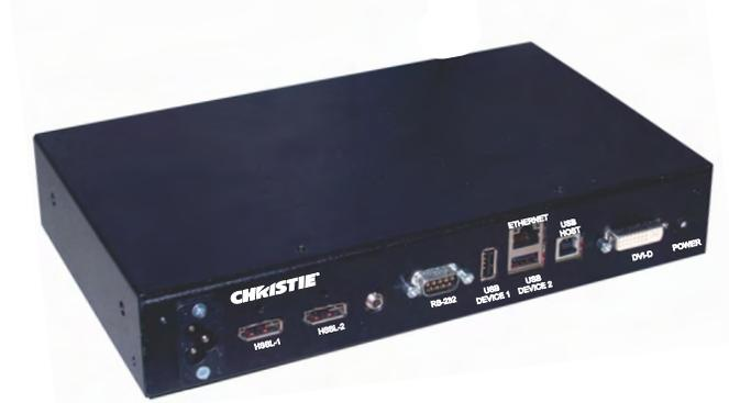
End users connect a PC or media player to the array using a DVI-D cable. The ECU then ensures the supplied video signal is properly displayed across the entire array. For more complex arrays, multiple ECUs can be used.
