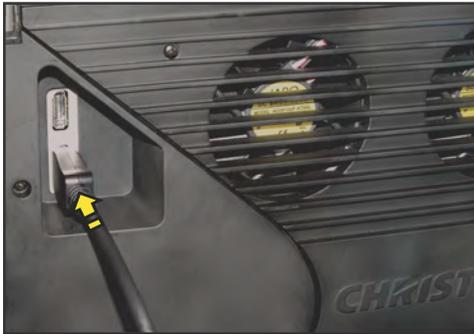
1. Plug the display port cables into either of the two ports on the back of the tiles.
