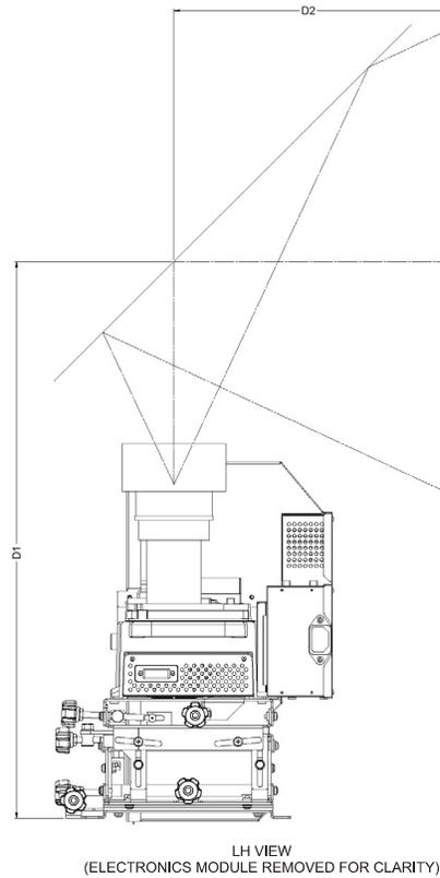
**FIGURE 2-8 THROW DISTANCE FORMULA FOR LENS-VERTICAL CONFIGURATION**
