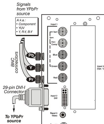
FIGURE 2-13 CONNECTING YPBPR
