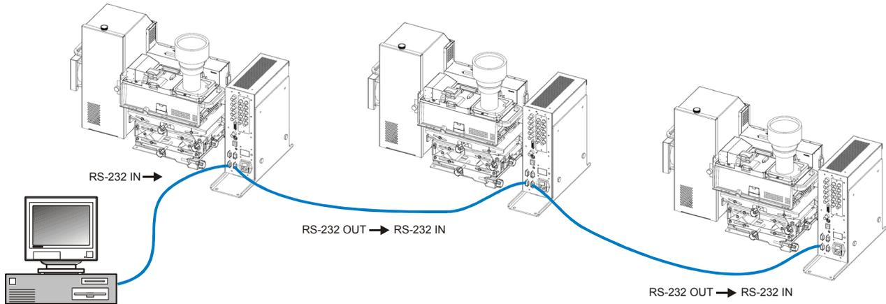
FIGURE 2-20 COMMUNICATING THROUGH RS-232
