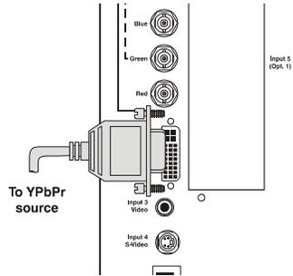
FIGURE 2-14 CONNECTING ANALOG OR DIGITAL VIDEO DEVICES
