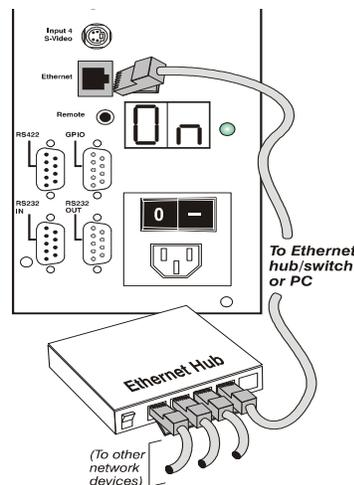
FIGURE 2-19 ETHERNET COMMUNICATION
