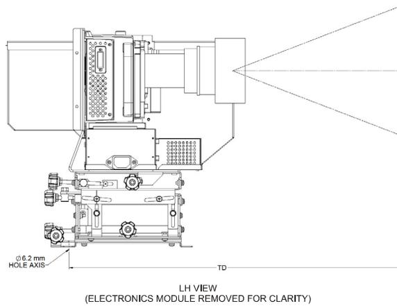
**FIGURE 2-7 THROW DISTANCE FORMULA FOR LENS-HORIZONTAL CONFIGURATION**
