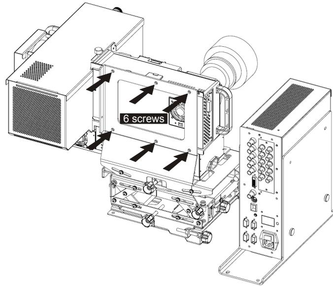
FIGURE 2-6 SECURE LIGHT ENGINE TO CONFIGURATION
