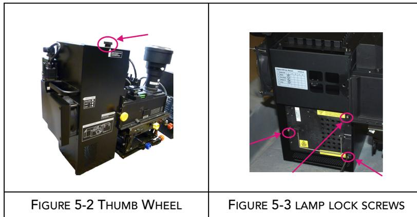
3. Loosen the (3) lock screws (*Figure 5-3*) on the lamp module held in the reserve position.
