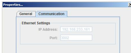
Figure 4-7 Properties Dialog Box, Communication tab Identifies the method used to connect the projector to the computer.
