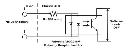
Figure 2-5 Inputs OFF State
