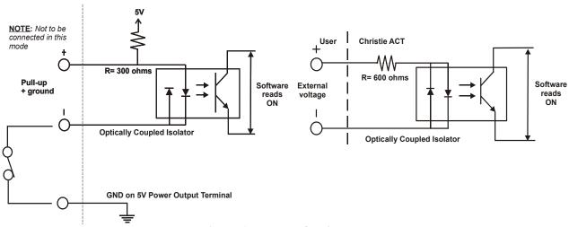
Figure 2-6 Inputs ON State
