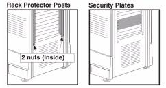
Figure 2-16 Remove Rack Protectors (2) and Remove Security Plates (2)
