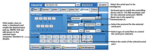
Figure 3-19 Config: Communication Tab
