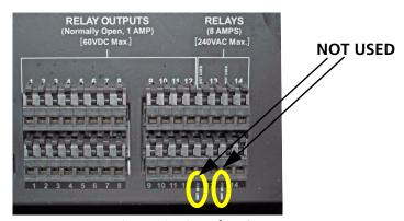
Figure 2-12 Relay Outputs
