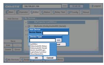
Figure 3-27 Adding a Device in the Editor: My Devices Tab
