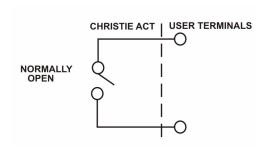
Figure 2-13 Relay Output
