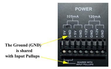
Figure 2-7 Inputs With Internal Pull-ups (Active)
