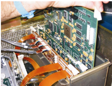
Figure 10 Insert new board
