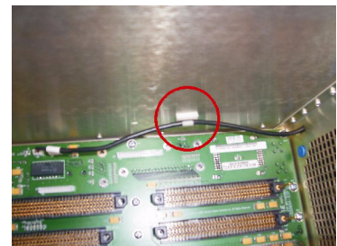
Figure 9 Attach clip and insert cable
