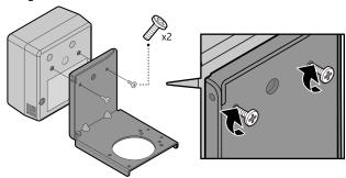
2. Align the holes on the camera bracket with the holes on the bottom of the projector and secure the camera to the projector with the two M3L8 screws.
