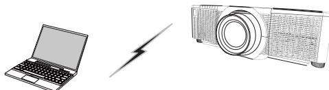
Fig. 3.3.a Without an access point communication (Simple Access Point)
