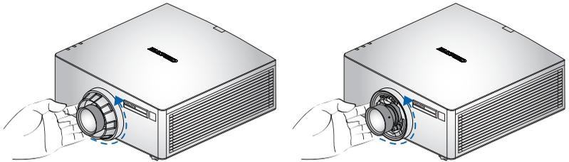
5. **Install the new lens:** Fully insert the lens assembly straight into the lens mount without turning. Rotate the lens cap clockwise to lock the lens in place.
